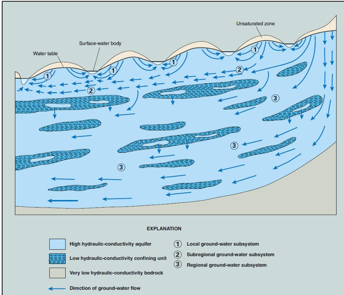
Figure 6: Groundwater flow systems (USGS, 1999)
